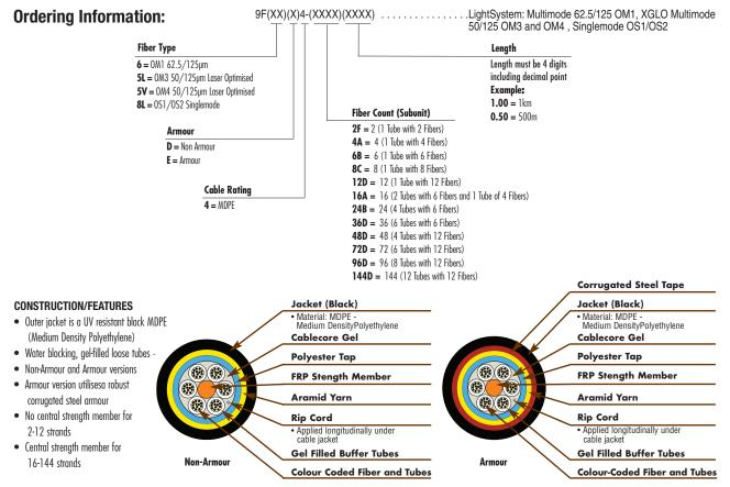
These cables provide a degree of rodent protection effective in many cases. The non-armour cable has a PE sheath which has a hard surface and provides a degree of rodent protection because it is disagreeable and unpleasant for most rodents to gnaw on. The armour cable has a PE sheath and corrugated steel tape which provides 100% rodent protection.
